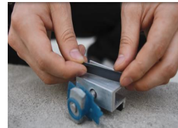
Fig. 3 – Sticking the rubber pad onto the clamp
