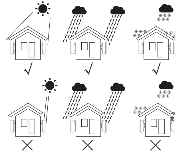
Figure 5.1 Recommended Installation locations
