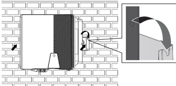
4. Check both sides of the heat sink to ensure that it is securely in place. insert one screw M5x12 each into the lower screw hole on both sides of the inverter anchorage bracket respectively and tighten them.
