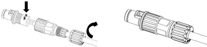
2. Remove the dust cap from the terminal of the meter connector, and connect the meter plug.
