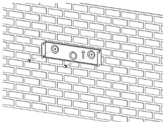
3. Position and hang the inverter onto the wall bracket ensuring the two studs located on the outer ribs of the inverter are slotted into the respective slots in the wall bracket.
