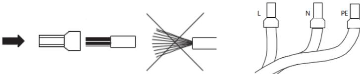
4. Insert the PE, N and L conductor through the AC connector housing and terminate them into the corresponding terminals of the AC connector terminal and make sure insert them
