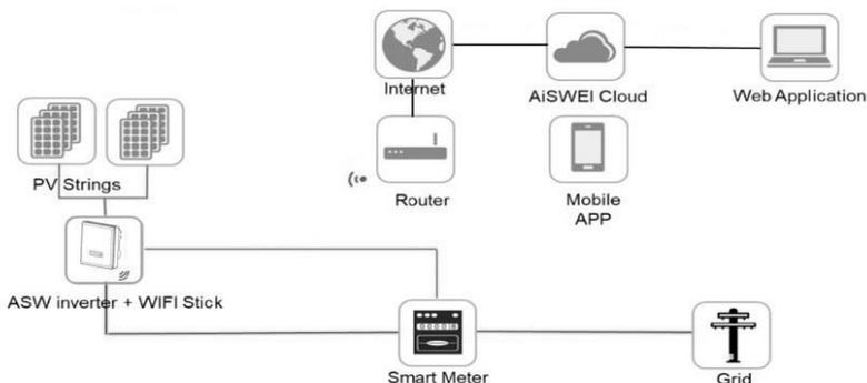
The smart meter should support the MODBUS protocol with a baud rate of 9600 and address set 1. Smart meter as above SDM630-Modbus connecting method and setting baud rate method for modbus please refer to its user manual.
