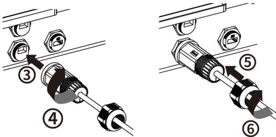
**Disassemble the network cable in reverse order.**
