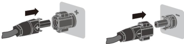
7. Ensure that all DC connectors are securely in place.
