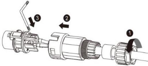
5. Connect the AC connector plug to the inverter's AC output terminal.
