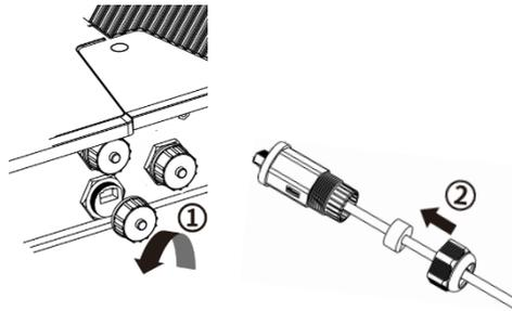
5. Insert the network cable into the corresponding communication terminal of the inverter according to the arrow sequence, tighten the thread sleeve, and then tighten the gland.
