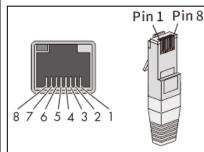
Pin 1=TX\_RS485A Pin 2=TX\_RS485B Pin 3=NC Pin 4=GND Pin 5=NC Pin 6=NC Pin 7=NC Pin 8=NC
